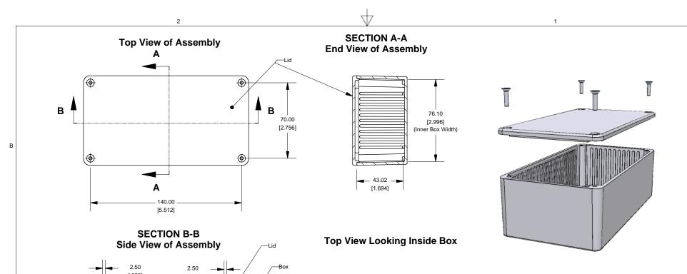
[.098] [.098] (Slot Width) (Post Width) 6-32 UNC - 2B ▼ 11.00 ∟ Ø3.50 ¥ 3.00 45.75 (Threaded Holes) [1.801] 50.50 (Inner Box Height) [1.988] [1.870] R4.00 [.157] 146.10 [5.752] 2.50 [.079] (Inner Box Length) 117.50 [.098] [4.626] 148.00 (Wall Thickness) [5.827]
